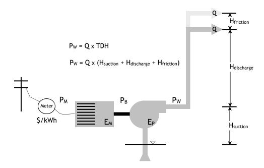
Pumping schematic ( $P_M$  = motor power;  $P_B$  = brake power;  $P_W$  = water power;  $E_M$  = motor efficiency;  $E_P$  = pump efficiency;  $H_{suction}$  = suction head;  $H_{discharge}$  = discharge head;  $H_{friction}$  = friction head; Q = pump flow rate and TDH = total dynamic head).
