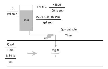
Generic graphic for setting up chemical dosing problems (AI = active ingredient, SG = specific gravity, CFP = chemical feed pump,  $Q_{CFP}$  = flow rate of chemical feed pump, and Q = process flow).
