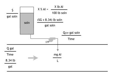
Generic graphic for setting up chemical dosing problems (AI = active ingredient, soln = solution containing active ingredient, SG = specific gravity, CFP = chemical feed pump,  $Q_{CFP}$  = flow rate of chemical feed pump, Q = flow (or volume) to which chemical is being dosed).
