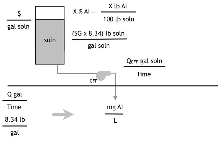
Generic graphic for setting up chemical dosing problems (Al = active ingredient, SG = specific gravity, CFP = chemical feed pump,  $Q_{CFP}$  = flow rate of chemical feed pump, and  $Q$  = process flow).
