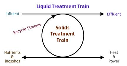
Generic WWTP graphic showing interaction between liquid and solids treatment trains, potential for resource recovery in the effluent, heat and power, and nutrients and biosolids outputs, and the potential impacts of recycle streams.
